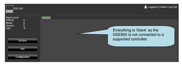
When connected to a supported controller, the initially displayed screen is a fully functioning SCADA display as shown and detailed overleaf.
